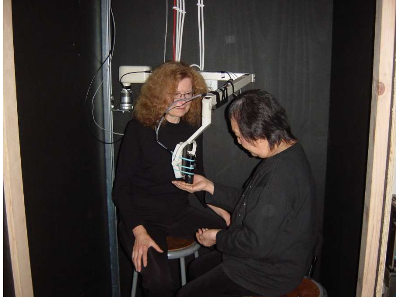
Figure 1. Rubik (left) making a simulated measurement with PMT placed on the palm of the hand of subject (right). Actual measurements are made in complete darkness.
