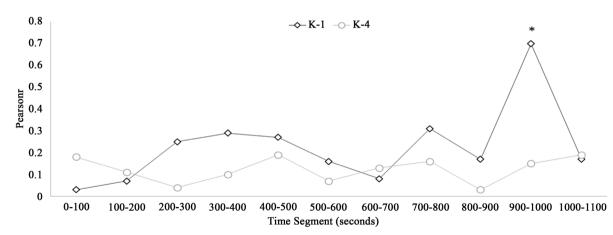
Figure 6. Correlation (absolute Pearson r) between pH values obtained within the two volumes of water for individual trials with Kp 24-Max of 1 (diamonds, K-1) and 4 (circles, K-4) when both beakers are exposed to the EMF sequences of the excess correlation protocol (Both On) as a function of time.
