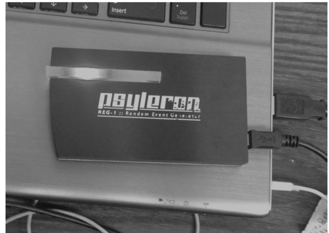
Figure 1. Random event generator (REG); Psyleron REG-1 device used throughout the following experiment.
