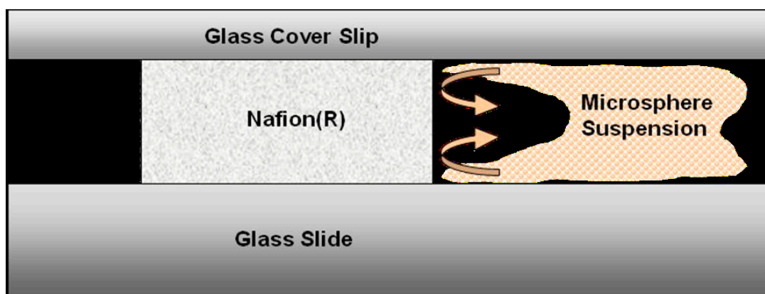
Figure 18. Schematic of cross section of microscope slide samples indicating the observed flow of microspheres that creates and maintains the EZ in the central focal plane of the sample.
