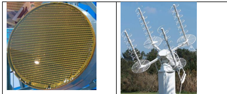
Fig. 3.1.1. Examples of engineering antenna arrays (taken from https://commons.wikimedia.org/wiki/File:PAK_FA_AESA_maks2009.jpg and https://commons.wikimedia.org/wiki/File:Traqeur_acquisition.JPG , permission is granted to copy, distribute and/or modify these documents under the terms of the GNU Free Documentation License).
