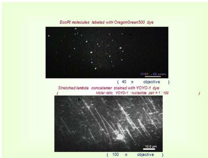
Figure 34. Fluorescent Image of EcoRI molecules and stretched DNA.
