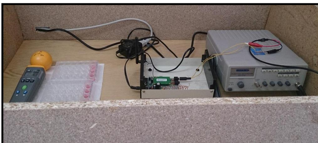
**Figure 1:** Wooden Chamber with RF System and the Instrumental Setup (from left to right: Electro Smog Meter, Plates, Horne Antenna, RF System, Function Generator).
