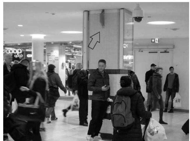
Figure 8. An example of highest exposure area. A man is standing with his smartphone just a couple of meters below a base station (see arrow). In that area maximum measured power density in the GSM +UMTS 900 downlink band was 95,544 \mu\text{W}/\text{m}^2 , which is the upper limit of measurement for EME Spy 200.
