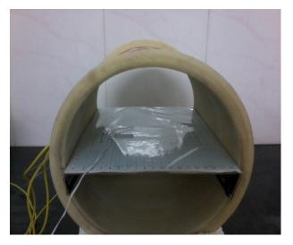
Figure 4: Homemade solenoid coils with calibrated plate. Digital thermometer probe located at the center of solenoid.
