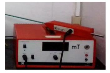
Figure 3: Teslameter and its probe
