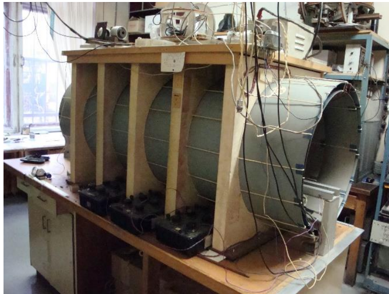
Figure 1. Experimental setup for shielding the geomagnetic field.
