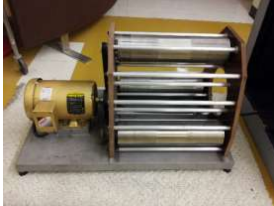
Figure 2: The ‘Resonator’ device with the soundproof cover removed. Shown is the motor drive system and motor belt (left) which rotates the three larger cylinders containing the magnets (right).
