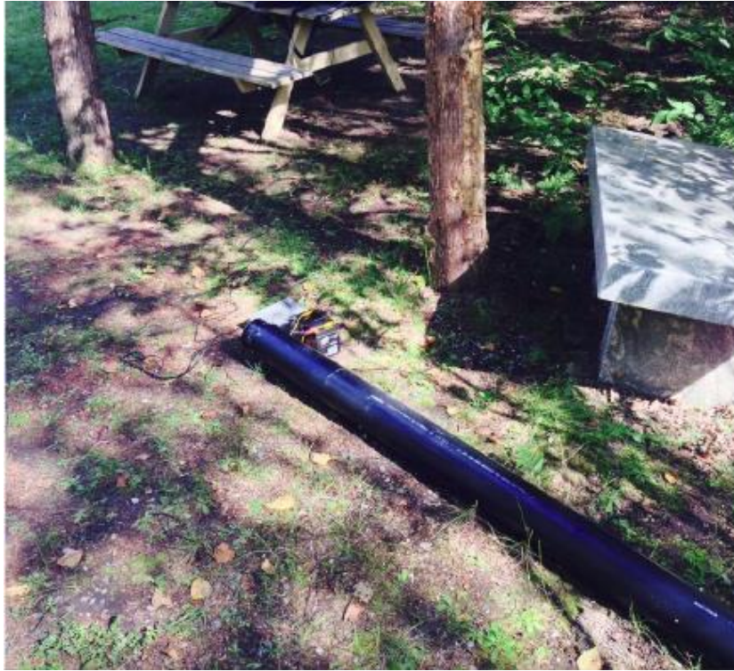
Figure 2. Cylinder containing the Schumann device “Herbert” by local Schumann resonances were measured.
