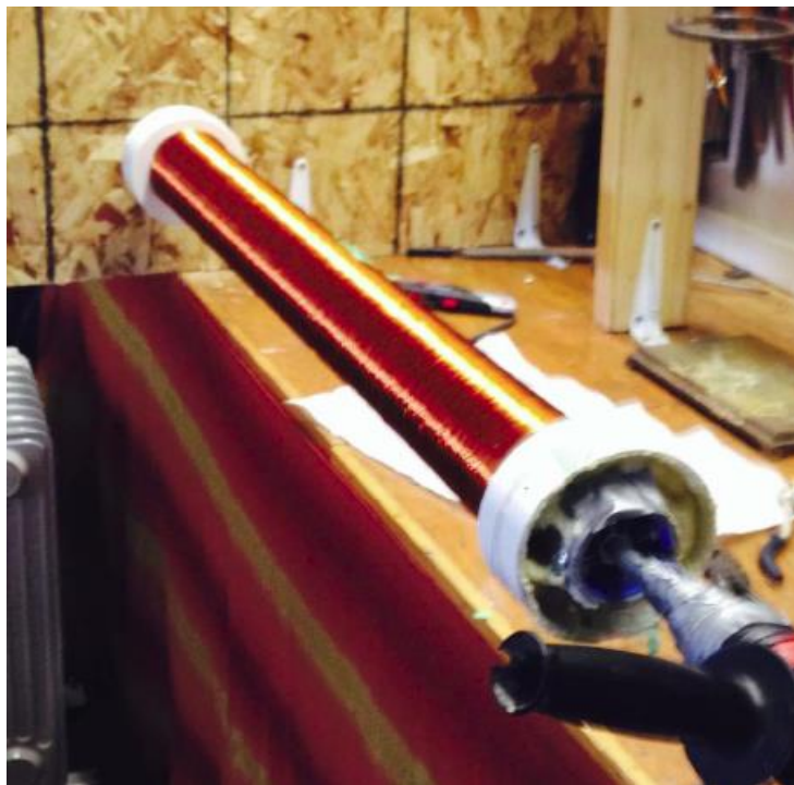
Figure 3. The Schumann (“Herbert”) unit during stages of wrapping the copper wire. There were between 96,000 to 97,000 turns.
