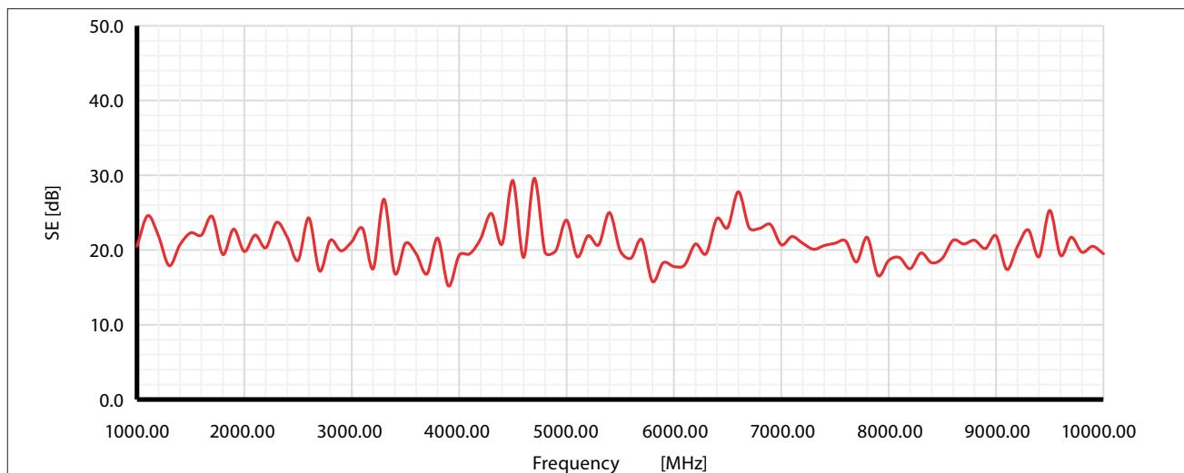
**Figure 4.** Shielding efficiency of fabric ADR TEX [dB] Vertical polarization
