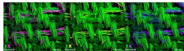
**Figure 1.** EDS imaging of carbon C in (Rayon, PA 66 and PES) and chromium Cr (magenta), iron Fe (yellow) and nickel Ni (blue) in ADR TEX shield
