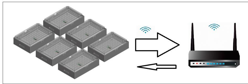
**Figure 7.** Schematic diagram of communication between ESP modules and the router
