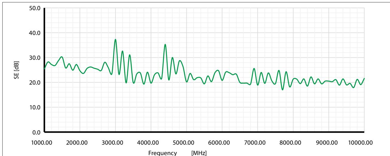
**Figure 5.** Shielding efficiency of fabric ADR TEX [dB] Horizontal polarization
