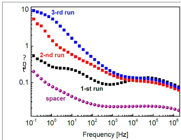
**Figure 3.** Room temperature frequency dependence of  $\tan \delta$  for a sample of ADR TEX shield placed between two dielectric spacers.  $\tan \delta$  dispersion of the dielectric spacer is also apparent
