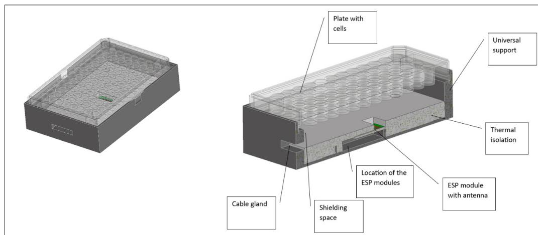
Figure 6. Designed experimental setup with universal support printed using PLA 3D printer
