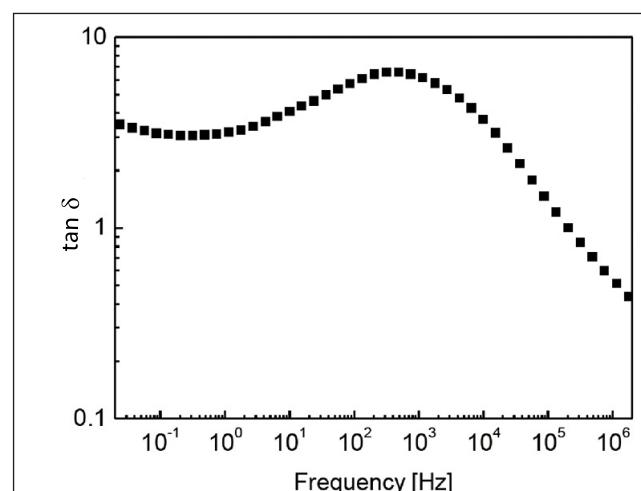
**Figure 2.** Room temperature frequency dependence of tan δ for a sample of Rayo/Nylon 55/45 fabric shield made with ADR Technology
